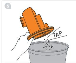
6 Dislodge any excess dirt by gently tapping the inner separator upside down above a bin.
