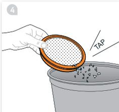
Tap excess dirt from the filter. Rinse under a tap and leave to dry for 24 hours.
