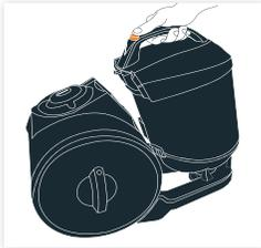
Remove dirt container by pushing down the dirt container release button and lifting the dirt container.
