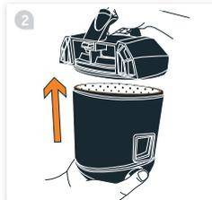
Lift the lid to reveal the pre-motor filter.
