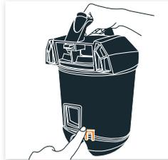
Hold the dirt container over a bin and press the dirt release latch (located at the rear of the dirt container).
