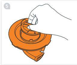
5 Remove the cap from the inner separator.
