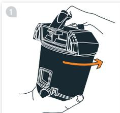
Hold the dirt container and twist the lid anti-clockwise.
