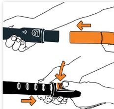
Slot the metal telescopic extension tube and hose handle together. All accessories can be fitted to the end of the metal telescopic extension tube and hose handle.
