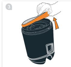
Lift out the pre-motor filter.
