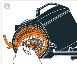
2 With the wheel cover off the post-motor filter is easily removed.
