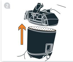
2 Lift the lid to reveal the pre-motor filter.
