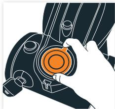
Adjust the power by rotating the dial for different surfaces as required.
