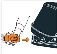
Insert the end of the hose into the unit. Ensure the hose has clicked into place.
