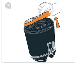
3 Lift out the pre-motor filter.
