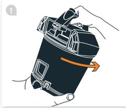
1 Hold the dirt container and twist the lid anti-clockwise.
