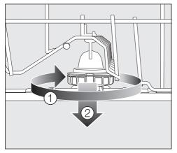
Rotate the screw thread of the middle spray arm clockwise (overhead perspective) ① (see diagram) and remove the spray arm ②.
