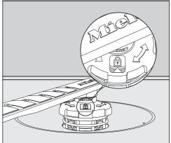
■ Rotate the screw thread clockwise until the arrow in the viewing window points to the lock symbol ⊕.
