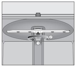
Push the upper spray arm upwards 1 to engage the inner ratchet. Then unscrew the spray arm by rotating the screw thread anti-clockwise (when viewed from below) 2.
