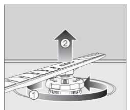
Rotate the screw thread of the lower spray arm anti-clockwise ① and pull the spray arm upwards to remove ②.
