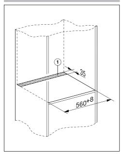
Create a cut-out ① in the interim shelf on which the steam oven is to be placed.
