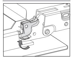
■ To relock the locking clamps, flip them back up to the horizontal position as far as they will go.
