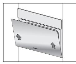
Hold the door on either side and evenly pull diagonally upwards from the hinge retainers.
