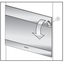
Insert the opener ① supplied about 3 cm into the gap between the door and the control panel on the righthand side and then pull the door open.
