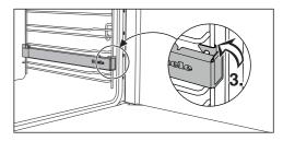
Then secure the telescopic runner to the bottom of the two rails as illustrated (3).
