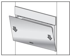
Hold the door securely on both sides and carefully fit it back onto the door hinge retainers. Make sure that you put the door back
