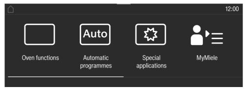
The menu path appears on the left of the **header**. The individual menu options are separated by a vertical line. ... I indicates that there are more options available, which are not visible because there is not enough space in the display.
