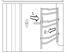
■ Pull the shelf runners out of the holder (1.) at the front of the oven and then pull them out of the oven (2.).
