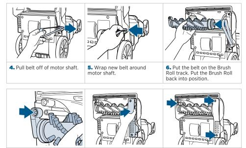
**7.** Align Brush Roll mount to<br/>screw post.**8.** Reposition belt cover.**9.** Reinstall 3 screws.
