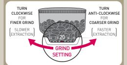
New Burrs are bedding in during the first few uses. The Grind Setting may require incremental adjustments before you reach your optimum espresso extraction.
