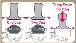
It is normal for the correct dose of coffee grinds to appear overfilled in the Filter Basket before tamping. Evenly tamp (press) coffee grinds to the level indicated.
