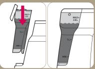
Fill with cold water from the tap and insert into position. For best espresso results, use room temperature filtered water.
