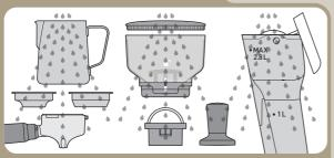
Wash the Milk Jug, One & Two Cup Filter Baskets, Group Handle, Bean Hopper, Top Burr, Tamper and Water Reservoir in warm water with a mild detergent. Rinse & allow thorough air drying.
