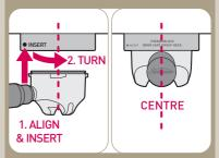
Keep Group Handle flat, align, insert & turn into Group Head. Group Handle should be in the centre position.
