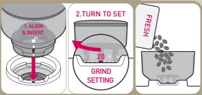
Insert & turn Hopper to set Grind Setting. As a starting point try Grind Setting 20.
