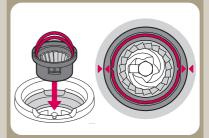
Use the two handles to insert Top Burr. Arrows should align when seated correctly. Place handles down, one on each side.
