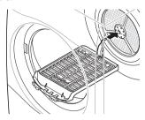
Place the drver rack on the structure above the lint filter and press it to complete assembly.
