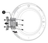
3 Remove the 3 screws from the door latch assembly **3** which is fixed between the door and the hinge assembly, and then remove the screw which is fixed on the door hook.
