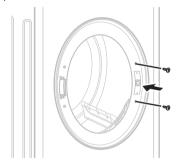
7 Install the door with the screws removed in step 1 and then check the door closes properly.
