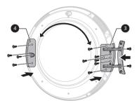
5 Remove the door catch **9** from the appliance frame by removing 2 screws and then assemble them on the opposite side.
