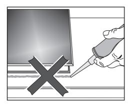
The SmartLine appliance and worktop may be damaged if the appliance needs to be removed after it has been sealed with a sealant.
