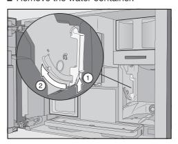
■ Press the button under the handle of the brew unit ① and, whilst doing so, turn the handle to the front ②.
