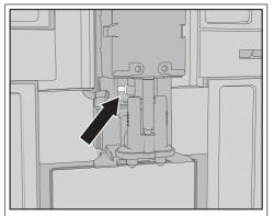
The connection piece in the milk pipework should not be removed. Clean the connection piece, if necessary, with the cleaning brush.
