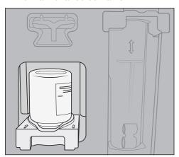
Pull the holder with the cartridge forwards and remove both. ■ Unscrew the cleaning cartridge from the holder. Dispose of the used cartridge with your household waste.
