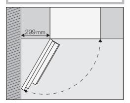
Check whether there is a gap of at least 299 mm between the wall or similar and the coffee machine so that the door can be opened wide enough to remove the bean container on the left (minimum door opening angle of 120°).
