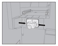
Push the catches on the left and right of the milk valve holder and pull the holder forwards to remove.
