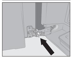
■ Remove the door opening limiters from the hinges by levering them out with a screwdriver, for example.
