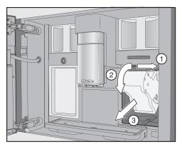
■ Pull the brew unit to the side ① first and then tilt to the front ②. Pull the brew unit forwards to remove it ③.
