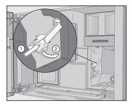
■ Press the button under the handle of the brew unit ① and, whilst doing so, turn the handle to the rear ②.
