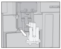
■ Hold the dispensing unit on either side and pull down to remove it.
