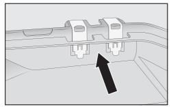
Clean the contacts (metal discs) and the space between them carefully, e.g. with a soft brush. Dry all parts thoroughly.
