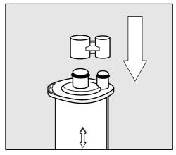
**Useful tip:** You can seal the descaling cartridge with the cap located on the cylinder of the cartridge. The cap can easily be released by snapping it off.
