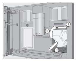
■ Pull the brew unit to the side ① first and then tilt to the front ②. Pull the brew unit forwards to remove it ③.
