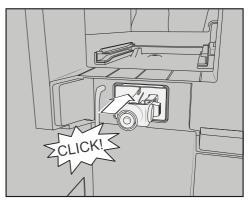
■ Fit the holder with the silicone seal until it clicks into position.
