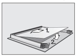
Refit the middle pane in such a way that the material number is legible (not reversed).
