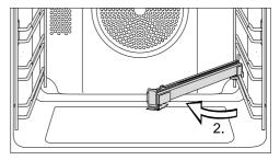
■ Then hold the FlexiClip telescopic runner at an angle in towards the middle of the oven compartment (2.).
