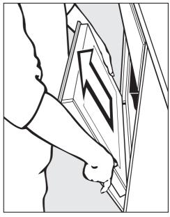
■ Hold the door on either side and pull it diagonally upwards from the hinge guides. Make sure that the door is straight.
