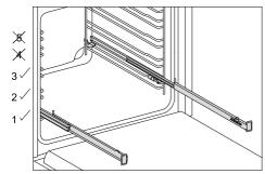
FlexiClip telescopic runners can only be fitted on levels 1, 2 and 3.
