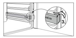
■ Then secure the FlexiClip telescopic runner to the lower rail of the shelf level as illustrated (3).
