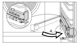
■ Then swing the FlexiClip telescopic runner back to the side and secure it to the top rail with an audible click (4).
