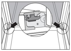
The oven door is connected to the hinges by retainers.
