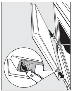
Hold the door securely on both sides and carefully fit it back onto the hinge retainers.
