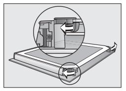
Flip the two glass pane retainers outwards to open them. To remove the inner panes:
