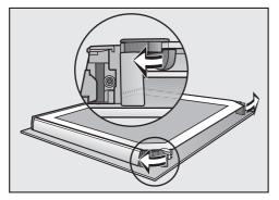
Flip the two glass pane retainers outwards to open them. You can now remove the inner pane and the two middle panes one after the other.
