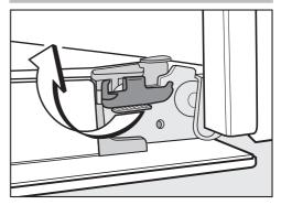
To relock the locking clamps, flip them back up into a horizontal position as far as they will go.
