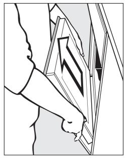
Hold the door on either side and pull it diagonally upwards from the hinge guides. Make sure that the door is straight.
