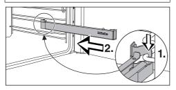
Hook the FlexiClip telescopic runner onto the lower rail of a shelf level at the front (1.) and push it along the rail into the oven interior (2.).
