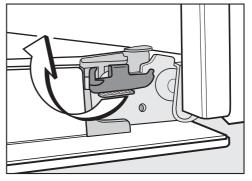
■ To relock the locking clamps, flip them back up into a horizontal position as far as they will go.
