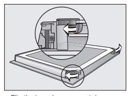
Flip the two glass pane retainers outwards to open them. You can now remove the inner pane and the two middle panes one after the other.
