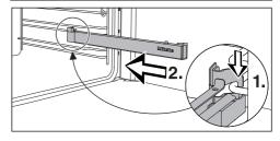
■ Hook the FlexiClip telescopic runner onto the lower rail of a shelf level at the front (1.) and push it along the rail into the oven interior (2.).
