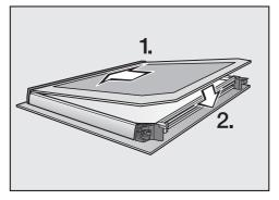
■ Push the inner pane with the matte printed side facing downwards into the plastic strip and place it between the retainers.
