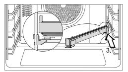
Slide the FlexiClip telescopic runner at an angle along the top rail as far as it will go (3).
