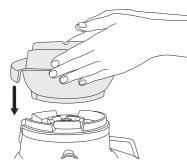
Align the arrows at the base of the stainless-steel filter basket with the arrows on the motor drive coupling and push down until it clicks into place to create a secure fit with the motor base.
