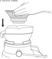
Place the juicer cover over the filter bowl surround, positioning the lower part of the feed chute over the stainless steel filter basket.
