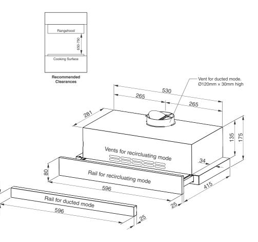
NOTE: The front rails are fitted with 4 screws behind the rail. -42mm rail to be fitted for ducted mode. -80mm rail to be fitted for recirculation mode.
