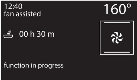
2. Press the control knob before the
