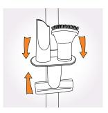
**NOTE:** For convenience there is a parking slot located at the rear of the vacuum cleaner where the floor head and tubes can be attached for storage and carrying.
