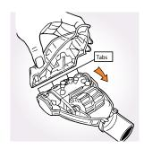
To re-assemble the TurboTool, ensure that the tabs are engaged and pivot the lower housing closed. Slip the locking ring over the neck of the TurboTool and into the groove to finish.
