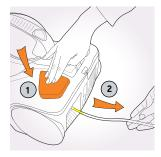
Fully unwind the power cord. A yellow mark on the cord indicates the recommended cord length. Do not exceed the cord length beyond the yellow mark.
