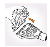
Detach lower housing and remove blockage.
