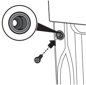
4. Cover the bushings using the covers that were previously removed.
