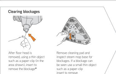
\*Ensure steam cleaner is completely cool before clearing blockages
