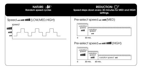
mode setting is selected, the tower fan is programmed to self-regulate through the various fan speeds. The NATURE mode is independent from the fan speed settings while the LED screen will still display the last selected fan speed setting.
