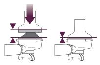
As a guide to dose, the top edge of the metal cap on the tamper should be level with the top of the filter basket AFTER the coffee has been tamped.
