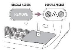
b) Use a flat-head screwdriver to rotate the right screw counter-clockwise until the valve is fully open. As the valve opens, steam may be released.
