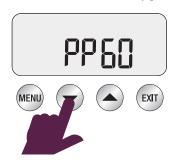
We recommend a range of between 55–65 as being optimum. Press EXIT to confirm setting and return to STANDBY mode.
