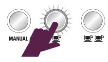
The machine will stop after 1 CUP volume has been extracted and will return to STANDBY mode.
