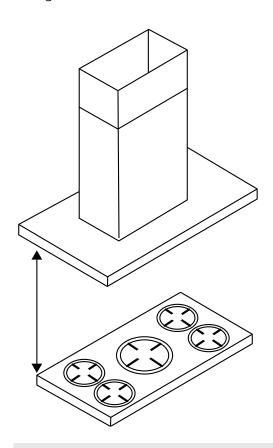
\*IMPORTANT: If the user decides to install the rangehood at a distance of less than minimum height above the cooking surface, Schweigen declines responsibility for damages suffered by the rangehood due to excess heat or damage to objects, people and others caused directly or indirectly by a malfunction, breakage or fire.
