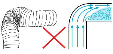
**1.** Crushed or kinked ducting creates sharp corners that creates turbulence. This reduces the size and efficiency of the ducting, lowers extraction and may cause excessive noise.
