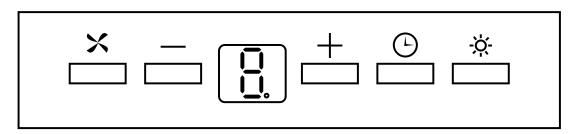
Press + to switch on the fan. The timer will only operate when the fan is switched on.
