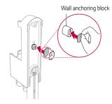
2 Use the remaining part of the tape to anchor the station to the wall before inserting the screw.
