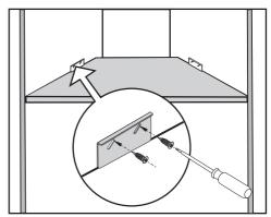
■ Secure the anti-tipping mechanism to the right and left-hand side walls of the housing unit with the 4 screws supplied (4 x 16 mm).
