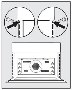
Open the door and use the screws supplied to secure the oven to the side walls of the housing unit through the holes in the oven trim.
