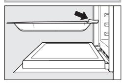
To remove the glass tray, lift it upwards slightly at the front when the safety notch connects with the sides of the oven.
