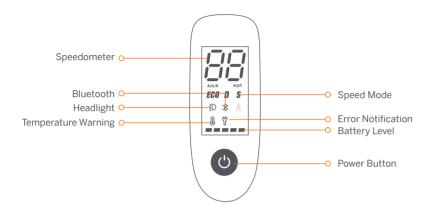
Power Button: Press the button to turn on; press and hold the button for 3 seconds to turn off. When the KickScooter is on, press the button to turn on/off the headlight and the rear light, and press twice to switch between the speed modes.
