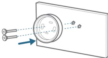
3. Firmly screw the base of the mounting bracket onto the wall. Fasten the ball knob of the bracket to the base of the bracket.
