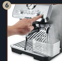
6 Push the STEAM button and let the steam flow out for a few seconds. Then push the button again. For optimal steam performance we recommend you repeat this action 3 or 4 times. This is to purge the steam arm before frothing or steaming your milk.
