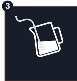
To make the froth, put the nozzle on the surface of the milk and air will catch by the mixing of milk and steam.
