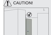
When you close the door, the vertical door strip on the left door should be bent inside (1).
