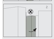
If you try to close the left door and the vertical door strip is unbent (2), you should bend it firstly, otherwise the door strip will hit the fixing shaft or right door. Thus a damage to the door slip or a leak will occur.
