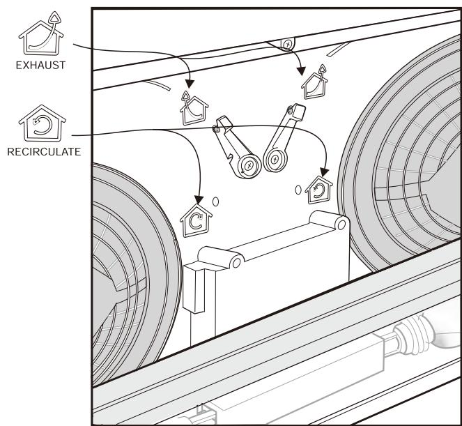
**IMPORTANT: SET CIRCULATING MODES BEFORE INSTALLING THE HOLE PLUGS.**
