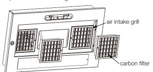
Optional carbon filters diminish cooking odours in the recirculated air. Depending on the frequency of use and the type of cooking, the expected life of carbon filters is 3 months. Using carbon filters will reduce the airflow of the rangehood.
