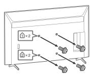
2 Attach the Wall-Mount Attachment (supplied with the TV) to the rear of the TV (to make it parallel with the wall).
