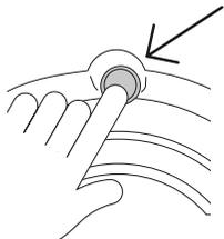
Cover the transit bolt holes with the plastic plugs delivered with the washer. Push to plug into place.
