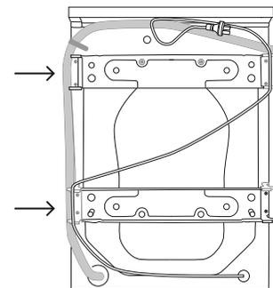
Detach the drain hoses from the plastic clasp, and remove the clasps on the side of the transit braces.
