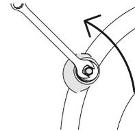
Use a spanner or socket to unscrew and remove all four transit bolts at the back of the washer.
