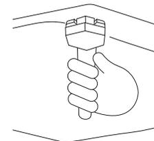
**Using the spanner provided, tighten the lock nuts against the base of the washer to lock the feet in position.**
