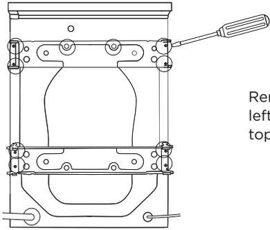
Remove the 10 transit brace screws from the left and right sides, and near the centre of the top brace.
