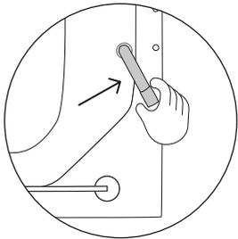
Pull out the two transit rods located below the two lower transit bolt holes.
