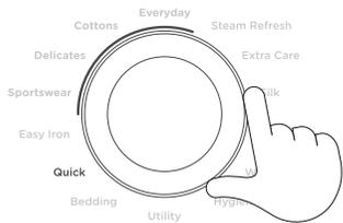
Select a **QUICK** cycle. Ensure the drum is empty and the door closed.
