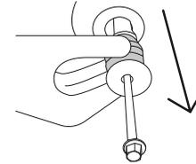
To remove the bolt, grommet and white plastic spacers, pull on the black rubber grommets.
