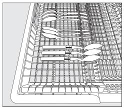
If spoon handles do not fit between the holders, lay them the other way round. You can push the left insert to the middle in order to accommodate tall items of crockery and long stemmed glasses in the upper basket (see "Upper basket – Loading the silicone elements of the FlexCare cup rack").
