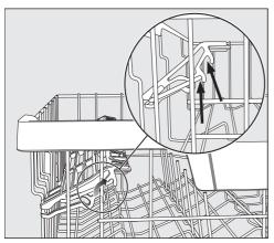
Pull the cup rack upwards and click it into the desired position (see arrows).
