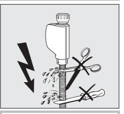
Risk of electric shock. There are electrical components in the water inlet hose.
