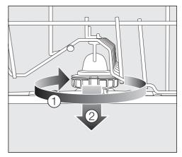
Rotate the screw thread of the middle spray arm clockwise ① (see diagram) and remove the spray arm ②.
