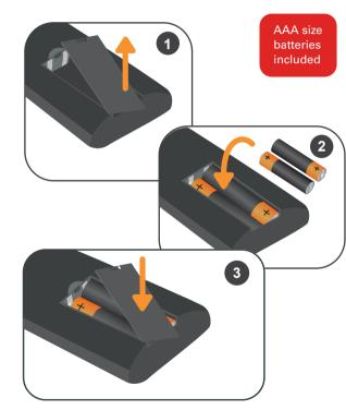
Image is for illustration purposes only. Position of battery cover/clip and polarities of batteries on your remote control may vary.
