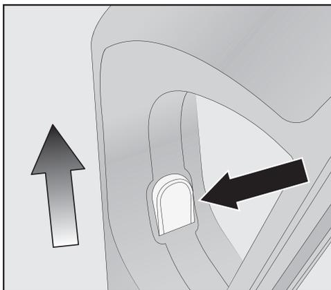
■ Press the release catch and remove the Comfort handle by pulling upwards.
