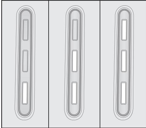
If the battery has not been used for a long time and has run down, it will go into a safe mode. As a result, the battery charging state indicator will only respond after approximately 30–60 minutes when charging in the PowerUnit.
