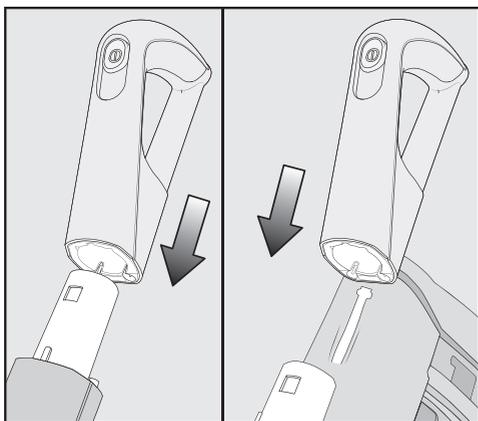
■ Push the Comfort handle down on to the suction tube connector from above until it audibly clicks into place (left image detail).
