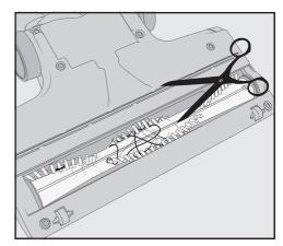
Cut any threads or hairs that have wound themselves around the roller brush with a pair of scissors. To guide the scissors, move along the guide track on the roller brush.
