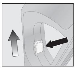
Press the release catch and remove the Comfort handle by pulling upwards.
