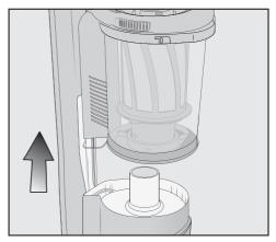
Lift the dust container upwards to remove it.
