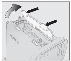
■ Press both release catches on the underside of the wall bracket and remove the cable compartment cover.
