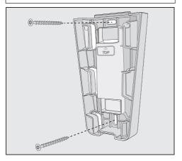
Attach the mounting plate to the wall.
