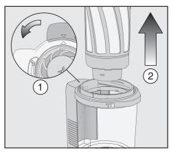
■ Empty the dust container over a bin and lift the pre-filter upwards to remove it.
