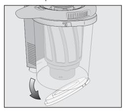
The cover at the bottom of the dust container will open and the dust will fall out.
