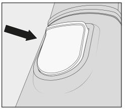
■ Press the release catch to separate the individual sections from each other.
