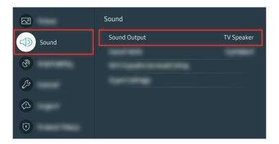
Check the volume on the screen. If a number for the TV volume is not displayed, select > Sound > Sound Output. Then, select TV Speaker.
