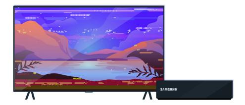
Check the antenna and input cable connections.
