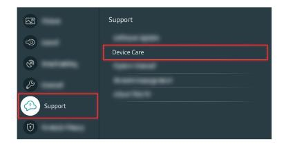
Go to (a) > (a) Settings > Support > Device Care > Self Diagnosis > Sound Test to check the sound.
