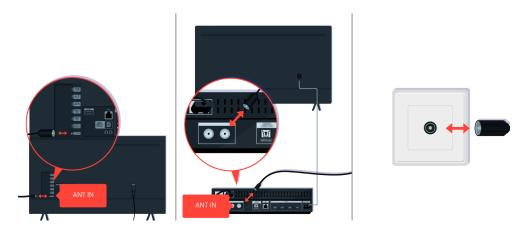
Check the antenna and input cable connections.
