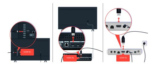
Check the antenna and HDMI cable connections.
