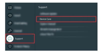
To check sound output, select (a) > (a) Settings > Support > Device Care > Self Diagnosis > Sound Test.
