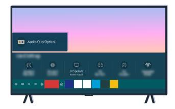
Check the volume on the screen. If a number for the TV volume is not displayed, select > Sound > Sound Output. Then, select TV Speaker.
